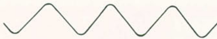
Fig. 8.2 Typical signal from a cassette recorder playing back the square wave shown in Fig. 8.1.
