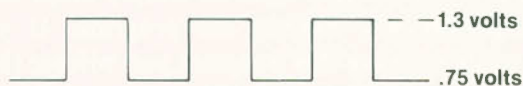
Fig. 8.1 The square wave sent to cassette line MIC from I/O port 254 by setting b3 alternately to 0 and 1.
